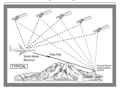
GLS approach procedures and techniques are identical to those of an ILS approach. GLS approaches are extraordinarily steady and smooth when compared with the current ILS system, even when critical areas necessary for the ILS approaches are unprotected during GLS approaches. There is no beam bending, no FM frequency interference, no interference from preceding aircraft, and no ground areas near the runway that need to be protected from surface traffic.
