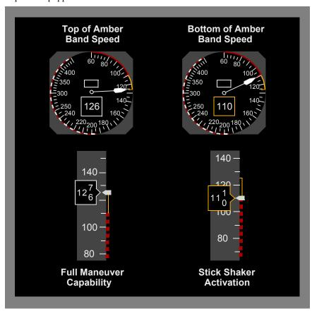
Minimum maneuver speeds (displayed as the top of the lower amber band) should not be confused with flap maneuver speeds. Flap maneuver speeds are based on airplane weight, while the minimum maneuver speed is calculated using airplane angle of attack and current airspeed. These speeds provide independent means to ensure that the current airspeed provides at least full maneuver capability for terminal-area maneuvering.
